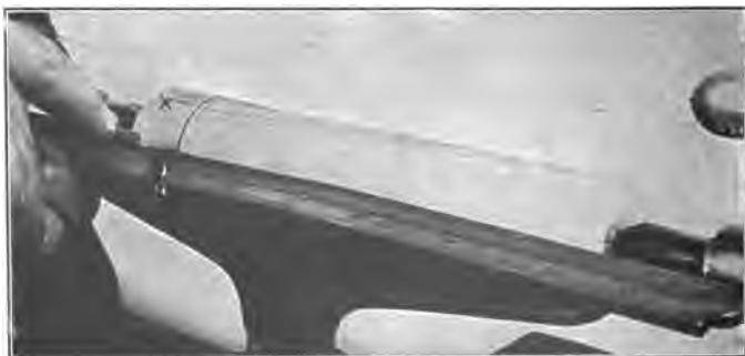
Fig. 19. Marking Spaces with a Pencil.
